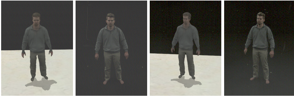
Figure 8: Confluent Motion enables creation of 3D videos with high-quality geometry models. Due to the accurate geometry the rendered appearance of the actor (left subimages) nicely corresponds to his true appearance in the real world (right subimages).
