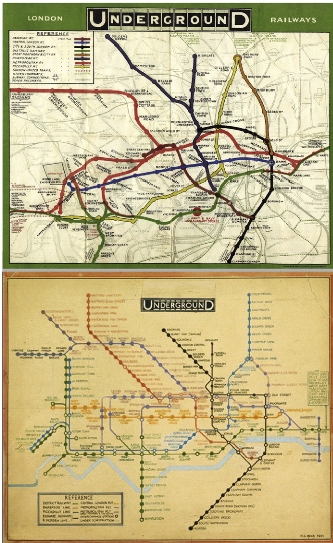
Fig. 1. Feature shift in London Underground maps. Top , first unified map of the London Underground from 1908 with the train lines subservient to the layout of the city. Bottom , lacking the recognizable geography, but maintaining the relative positions and connection points, the revolutionary 1931 design by Harry Beck.
