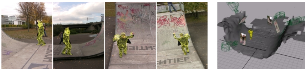
Figure 26.2: Tracking of a person in an outdoor scene with 4 moving cameras: pose result at one time instance overlaid into the 4 camera views (left) and reconstruction of the of the scene, including the camera motion, static scene background, and the tracked person (right).
