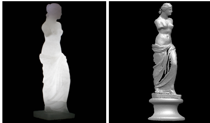
Figure 30.30: By combining phase-shifting and polarization our method faithfully captures the 3D geometry of very translucent objects such as this alabaster Venus figurine (height \approx 19\text{cm} ).
