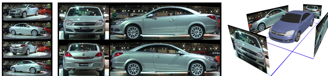
Figure 26.1: Left to right: frames from the input video sequence; ortho-images that are automatically assembled out of a large number of different input frames; final model that is modeled manually in a 3D modeling package by using the ortho-images as blueprints.
