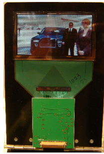
Figure 28.12: This is a demonstrator fabricated by TDK using a display driver based on our algorithm.
