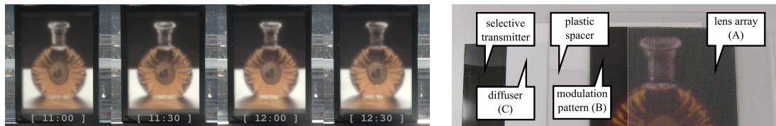
Figure 30.35: A 4D Passive Reflectance Field Display: mounted to a window in daylight (left), it renders a scene in the outside illumination. As time progresses, and the sun traverses the sky, highlights and shadows move naturally in the generated image. The embedded construction consists of few off-the-shelf components (right).
