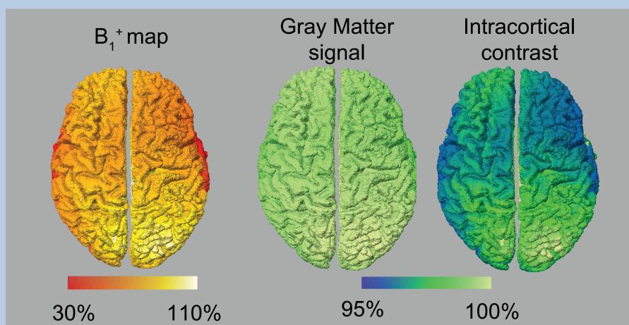
To assess the quality of the T1 maps, we also acquired a whole brain B<sub>1</sub>+ in one subject [5] and simulated the effect of B<sub>1</sub>+ variation on the MP2RAGE ratio-image signal in Matlab based on analytical equations for the MP2RAGE [1,6] and MR tissue values at 7T [7]. Despite large B<sub>1</sub>+ variations, the estimated gray matter signal and intracortical contrast was very homogeneous.
