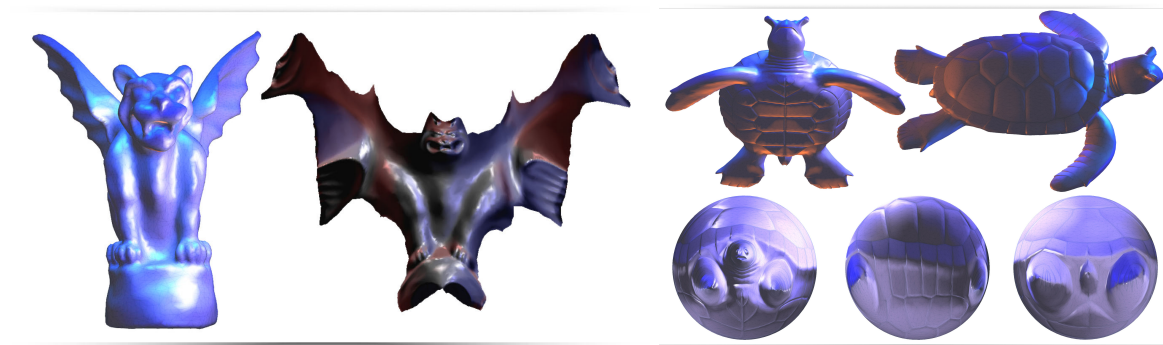
Figure 15.2: The left pair of images shows a free boundary planar parameterization of a gargoyle model. The right pair of images shows the spherical parameterization of a turtle model. Both results illustrate the robustness and low distortion qualities of the proposed methods.
