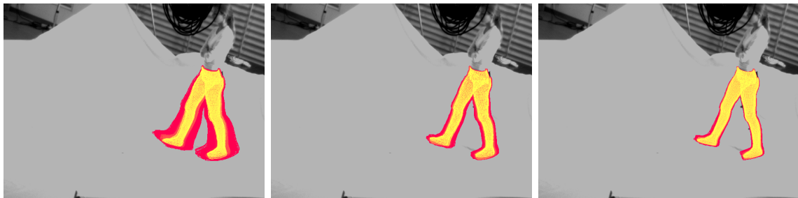
Figure 15.20: Particles with a higher weight are brighter, particles with a lower weight are darker. The particles converge to the pose with the lowest energy as the number of steps increases.
