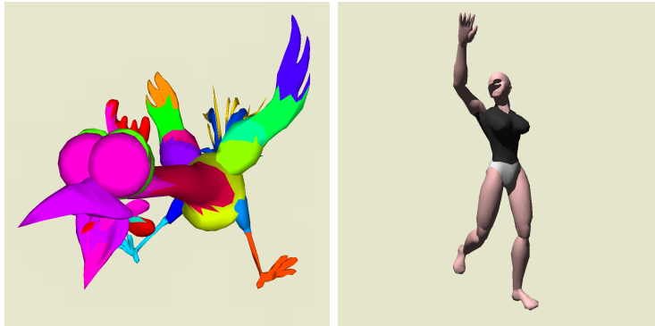
Figure 15.39: Left: The CHICKEN animation ray traced in realtime. The color encodes separated clusters generated by our motion decomposition algorithm. Right: The CALLY example scene demonstrating interactively skinned meshes with ray traced shadows at 1024 \times 1024 pixels on a single CPU.
