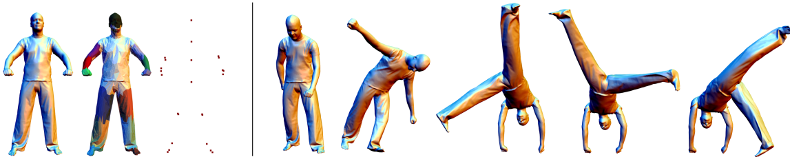
Figure 15.5: Example of a deformation of a scanned model based on a set of markers from an optical MoCap system.
