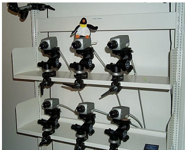
Figure 8.25: The Lumi-Shelf, consisting of six FireWire cameras mounted in a bookshelf.
