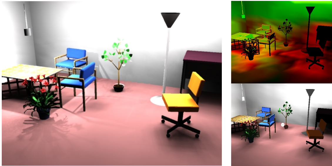
Figure 10.40: Left: Result of the final gather step. Right upper small image: number of samples (red: visib., green: formfactor). Lower small image: radiosity solution.
