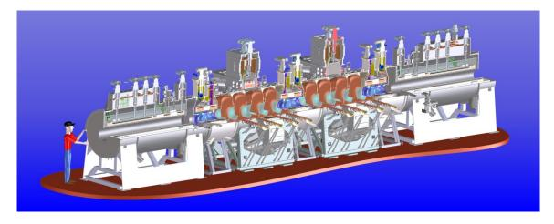
Figure 11: Engineering drawing of the MICE experiment [16]. The central region shows two ionization cooling cells, with instrumentation regions on either side for measuring the parameters of muons entering and leaving these cells.
