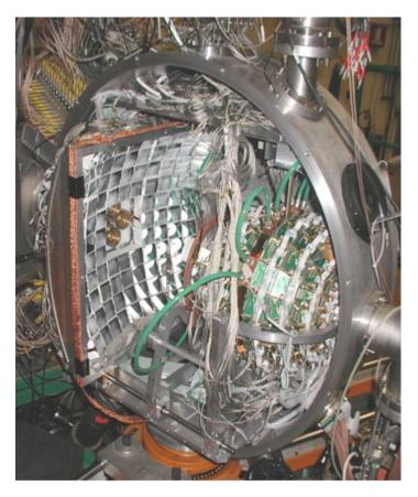
Figure 15: The  $8\pi LP$  experiment used for measurement of the  $^7Li(d,p)^8Li$  cross-section.
