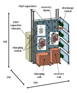
Figure 5: Design of the pulsing system for the Super Beam horns.
