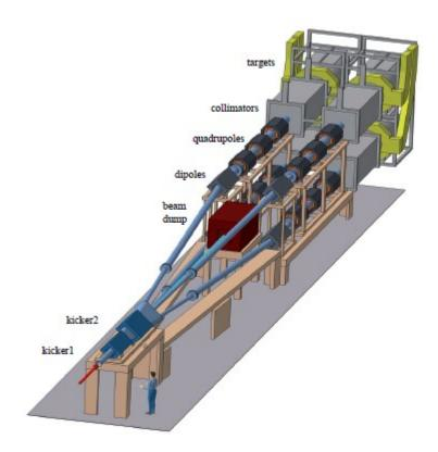
Figure 2: The Super-Beam beam transport and distribution system.
