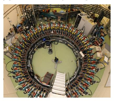
Figure 13: The EMMA proof-of-principle accelerator at the Daresbury Laboratory.
