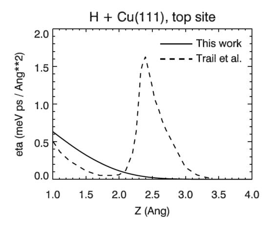
S7. Friction coefficients computed for motion of H along a line that is perpendicular to a Cu(111) surface, and goes through the top site on that surface. Results are shown for the LDFA method <sup>48</sup> used in this work and for the method used by Trail et al. <sup>53</sup>.
