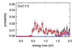
S6. Total energy (adiabatic + non-adiabatic) loss distributions for 5 eV H-atoms scattered from Au(111) and Cu(111) at the indicated incidence angles ,  $T_S$ =120K.
