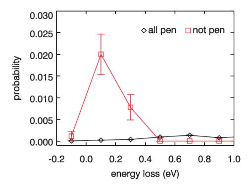
S5. The angularly resolved energy loss distribution is shown for scattering of 5 eV H atoms from Au(111) at  $\theta_i = 60^\circ$  and  $\phi_i = 0^\circ$  to  $\theta_f = 60^\circ$  and  $\phi_f = 90^\circ$ , at  $T_s = 120$  K. In contrast to Fig.4, here a contribution has been taken into account from H-atoms that scatter with penetration at times longer than the timescale of our simulation.
