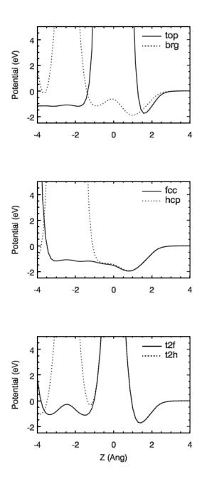
S3. The H-surface interaction potential is shown as a function of the atom-surface distance Z in Å, for H +Au(111) (see also Fig.S1).
