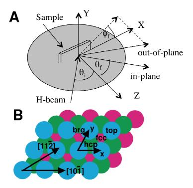
S1. Definition of incidence angle  $\theta_i$ , and scattering angles  $\theta_f$  and  $\phi_f$  (A). Plot of the (111) surface of fcc metals like Cu and Au (B). Indicated are the high symmetry sites top, hcp, fcc, and bridge (brg). Also indicated are the crystallographic directions corresponding to the two planes of incidence studied in this work.
