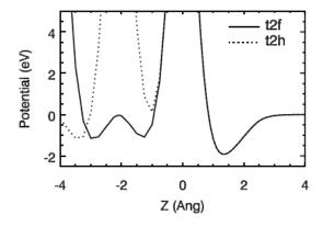
S2. The H-surface interaction potential is shown as a function of the atom-surface distance Z in Å, for H + Cu(111) (see also Fig.S1).
