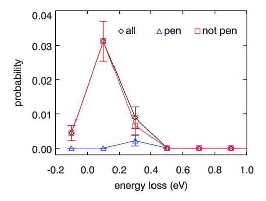
S4. The energy loss distribution for specular scattering is shown of H-atoms that have scattered from the surface ("all"), that have scattered from the surface with penetration of the surface ("pen"), and that have scattered from the surface without penetration of the surface ("not pen"). Results are shown for an incidence energy of 5 eV, for H + Au(111) and  $\theta_i = 60^\circ$  and  $\phi_i = 0^\circ$ .
