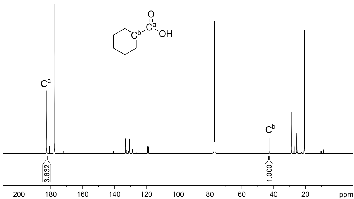
Figure S4.4. Quantitative ^{13}\text{C} NMR spectrum of the reaction mixture after the catalysis indicating the ratio of the integrals for \text{C}^a:\text{C}^b . Measured in \text{CDCl}_3 at ambient temperature with a resonance frequency of 151 Mhz.
