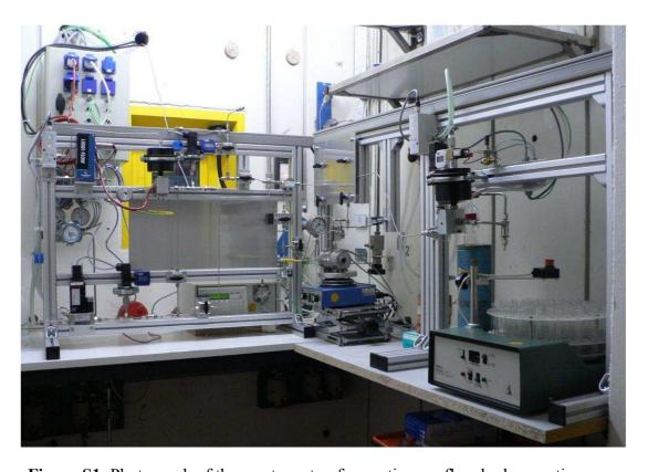
Figure S1: Photograph of the reactor setup for continuous flow hydrogenation
