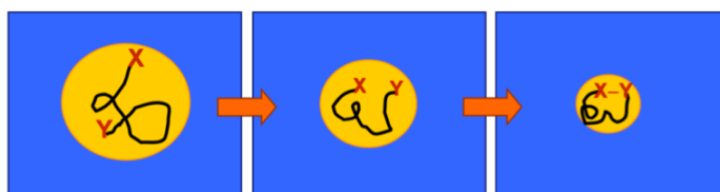
Figure 1.27 Intramolecular reaction of a separated polymer chain in a miniemulsion droplet during the evaporation of the solvent. 72
