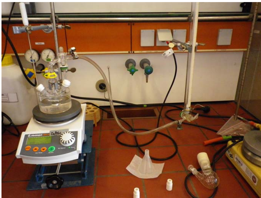
Figure S4: Picture of experimental setup including three-necked flask and gas burette.
