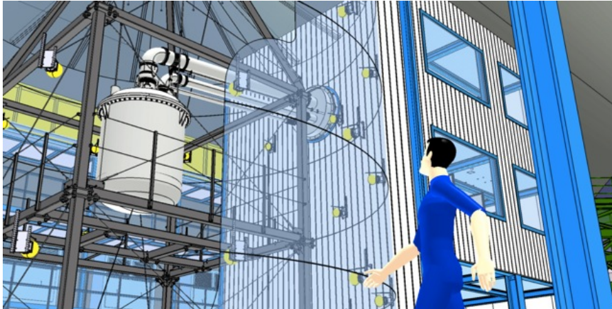
Figure 1.10: Artist's view of the XENON1T cryostat inside its 9.6 m diameter water shield and Cherenkov muon veto.
