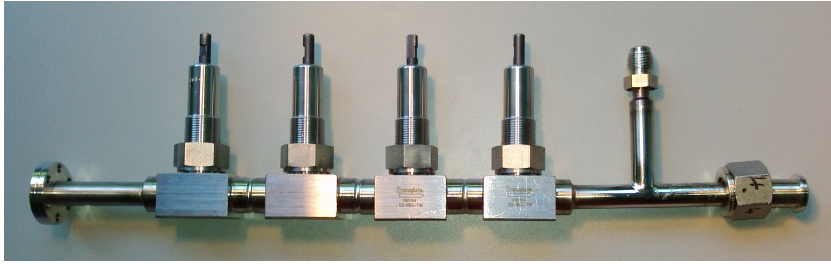
Figure 3.17: Employed vessels (xenon sampling device) for xenon samples. The four (fully metal sealed) valves enclose three volumes of \sim 10\text{ cm}^3 size. The port to the left is used to connect the xenon sampling device to the PCGC, while the two flanges to the left are used to connect the xenon sampling device to the vessel that contains the xenon and to install a vacuum system during preparation.
