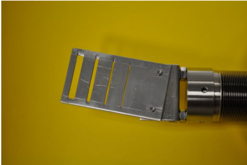
Figure 3.5: Visible are the four slits with dimensions (from left to right 4,2,1 and 0.6 mm) \times 20 mm mounted on a translation stage. The slits are inserted under an angle, since the flange where it is meant to be installed also has an angle corresponding to the laser beam. This angle is crucial for Doppler effect measurements (See Section 4.1).
