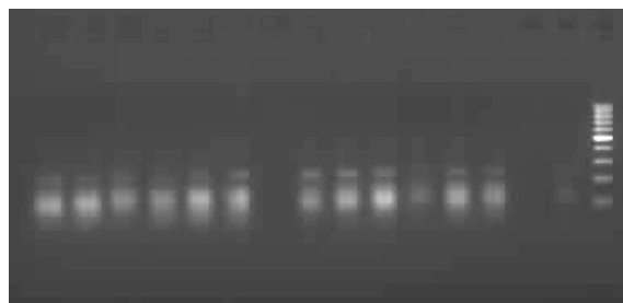
Figure 2. PCR amplification check on 1.8% agarose gel. Lanes 1-15 represent PCR products (with a couple of failed amplification on lane 7 and 14), lane 16 represents 100bp DNA marker.
