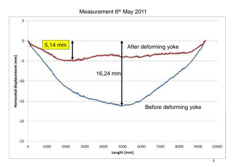
Figure 23. Position of the beam pipe axis along the magnet.
