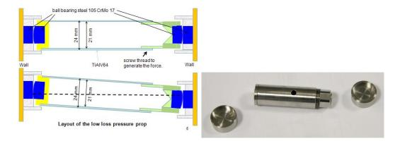
Figure 25. Principal layout of a pressure prop with low thermal conductivity and the first prototype.
