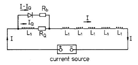
Figure 32. Schematics of the HERA quench protection.
