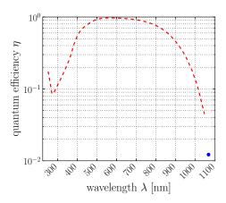
**Figure 18.** Measurement of the quantum efficiency of the PIXIS 1024B: The dashed line is the quantum efficiency measured at a temperature of T=25 °C taken from the data sheet [100]. The single bullet is the measurement of the quantum efficiency at T=-70 °C.
