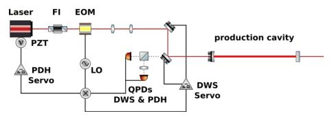
Figure 8. Schematic of the ALPS-II injection stage including the production cavity.
