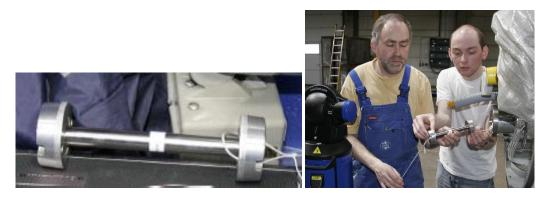
Figure 30. The "mouse" survey tool, used to measure the position of the middle of the beam pipe along the magnet.
