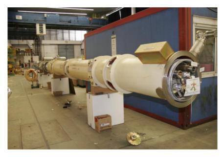
**Figure 22.** Setup of a HERA dipole to test the deformation method. The dipole was used as an exhibit for many years and was not foreseen as a spare for HERA.
