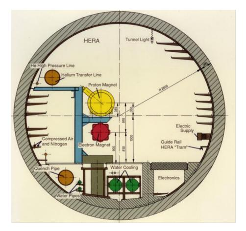
**Figure 34.** Cross section of the HERA tunnel in the arcs. The ALPS-IIc setup in the straight sections of the HERA tunnel will look very similar, the main difference being that the components of the HERA electron ring will have been dismantled.
