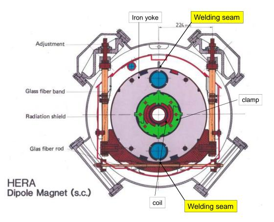
**Figure 20.** Cross section of the HERA dipole cryostat. The welding of the half cylinders of the Helium vessel around the iron yoke was performed in a big tool which forced the cold mass to a given curvature. The beam pipe was forced to follow the curvature by spacers glued to the outside of the pipe.
