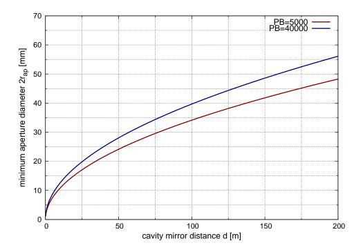
**Figure 9.** Minimum aperture diameters  $2 \cdot r_{ap}$  required to allow for a power buildup of 5000 for the PC (red, lower line) and 40000 for the RC (blue, upper line) plotted over the cavity mirror distance *d*. Additional mirror losses of 8 ppm are assumed for each cavity mirror.
