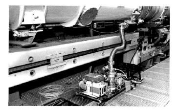
Figure 39. Turbo-molecular pump station.
