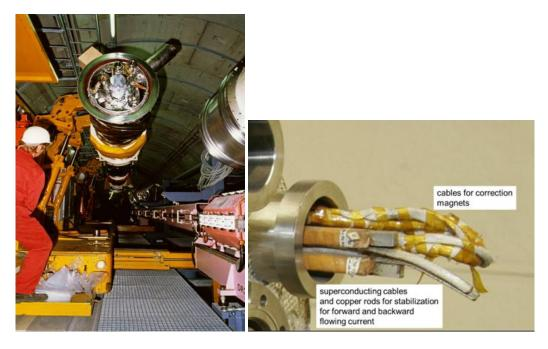
Figure 46. HERA tram (left) and superconducting cables in 4K Helium tube (right).
