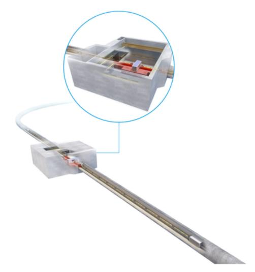
**Figure 6.** Artist's view of the ALPS-IIc setup. The picture shows a straight section of the HERA tunnel equipped with 20 HERA dipoles. The middle part, accommodating the central breadboard including the "wall" is highlighted.
