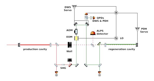
Figure 11. Schematic of the ALPS-II regeneration cavity including control loops.
