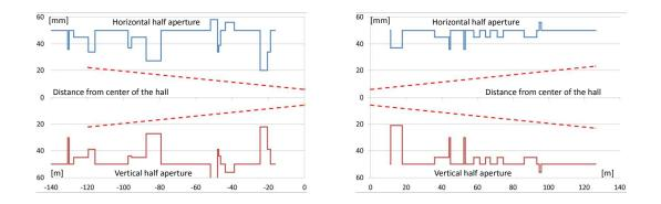
**Figure 44.** The figure shows the horizontal and vertical apertures of the proton beam pipe to both sides of HERA hall west. The Gaussian laser beam with a size required for a power buildup of 40000 is sketched as a red dotted line. As can be seen there is ample space to accommodate the laser beam on both sides.
