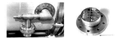
Figure 38. Pumping port with rupture disk.
