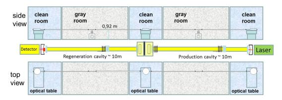
Figure 13. Experimental setup for ALPS-IIa in building 50 room 607.
