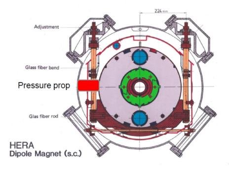
Figure 24. Position of a pressure prop in the dipole cryostat.
