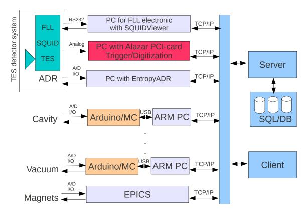
Figure 43. Scheme of the distributed data acquisition and control system.
