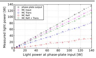
FIG. 4 (color online). Measurement of the light power at different locations in the setup as a function of the injected laser power. Statistical uncertainties in the measurement data are smaller than the marker's size and here not reported. Systematic errors in the calibration of each power curve are of order 5%.
