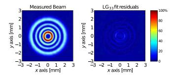
FIG. 5 (color online). Intensity profile of the 83 W  $LG_{33}$  beam transmitted by the MC cavity (left) compared with fit residuals (right). Maps have same units and scale.
