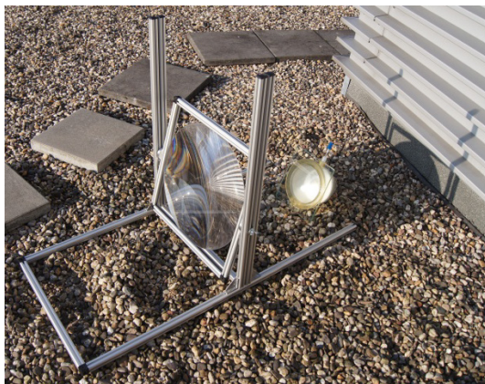
Figure 68: Full reaction setup with Fresnel lens and the modified desiccator.
