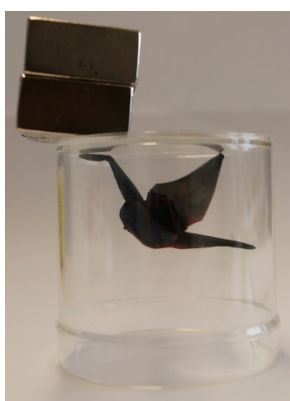
Figure 52: The magnetic cranes are easily lifted up and kept afloat by a permanent magnet.
