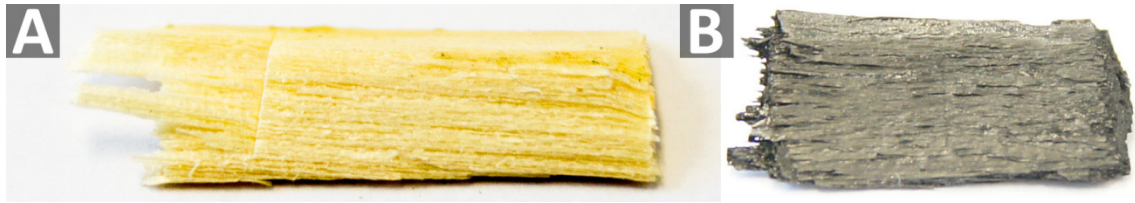
Figure 72: Wood samples A: before (not soaked) and B: after calcination.
