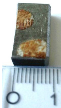
Figure 76: Example of a scrap metal specimen after cutting.
