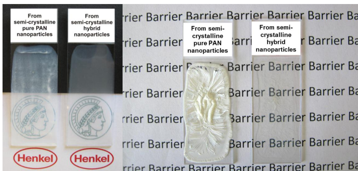
Figure 38. Photographs of semi-crystalline films derived from PAN and PAN/methacrylic polymer hybrid dispersions. The films on the left were prepared by rod-coater, while the films on the right were prepared by direct deposition of 1.5 ml dispersions from pipettes. PAN is accounted for 30 % in composite film based on total dry weight.
