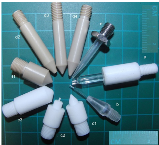
Fig. 3. Capillaries of different material, tip size and geometry; a – glass with PTFE mounting (ID 500 \mu\text{m} ), b – glass with PE mounting (ID 100 \mu\text{m} ), c1 to c3 – PTFE of different tip shape and size (200–800 \mu\text{m} ), d1 to d4 – PEEK of different tip size (ID 200 \mu\text{m} to 800 \mu\text{m} , d2 is a composite designed tip with steel ring inside), e – PE tip with steel mounting (ID 450 \mu\text{m} ).
