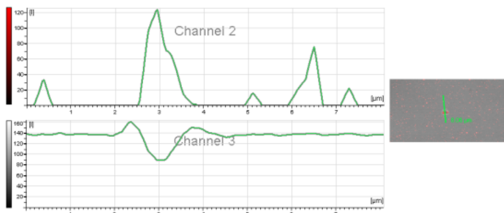
Figure 4.18: Overlay micrographs (right), fluorescence intensity profile (left red scale) and transmission intensity profile (left grey scale) of vesicles formed by PB_{80}(Glc)-b-PNIPAM_{557} with encapsulated Rhodamine B.
