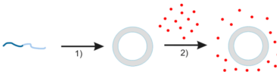
Figure 3.12: Preparation of the sample for the "visualization" of the external block by SERS. Step 1) is the dissolution of the polymer followed 2) by addition of colloidal gold.
