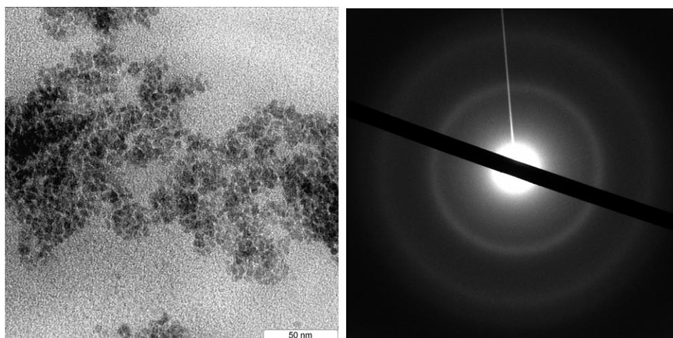
Fig. 8. A TEM image and a SAED pattern from a solution of mixed Na<sub>2</sub>S- and CdCl<sub>2</sub>-loaded vesicles not subjected to electrofusion. The reagent concentration in the vesicles was 0.3 mM. Only irregular sediments with poor crystalline structure are formed due to vesicle rupture upon deposition on the TEM grid and subsequent content mixing.
