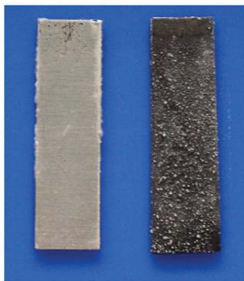
Fig. 5 Long-term corrosion test: Al alloy covered by polyelectrolyte/inhibitor (left) and unmodified Al plate (right). (Reprinted with permission from Andreeva et al. 23 © 2008 Wiley-VCH.)
