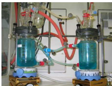
Figure 42: Set-up for the chemical polymerization using FeCl 3 as oxidant and HCl as dopant. The reactors are equipped with a thermostatted jacket and an air-tight seal allowing the reaction to proceed at a controlled temperature and in an inert atmosphere.
