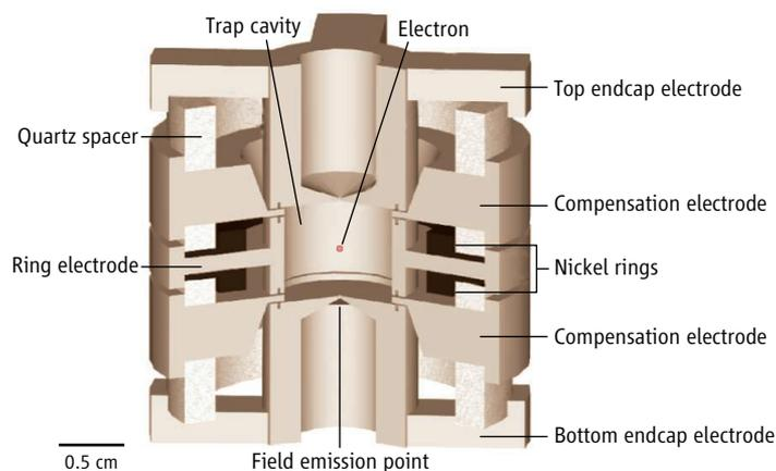
**One-electron cyclotron.** A magnetic field along the axis confines the electron radially; an oscillating electric field applied to the endcap electrodes confines it longitudinally. Nickel rings slightly perturb the magnetic field so as to couple the radial and longitudinal motions. The electron is trapped in a cavity that inhibits spontaneous emission. Other electrodes are used to control the electric field so as to reduce QED effects of the vacuum.
