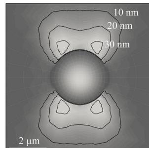
The [101] indentation axis was found to be characteristic for the easy activation of ordinary dislocations. In comparison to the known fcc pile-up shape the  $\gamma$ -TiAl pattern exhibits pronounced piling up in the slip directions of ordinary dislocations.
