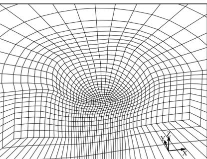
Discretization of the indentation process into 15060 hexahedral finite elements.
