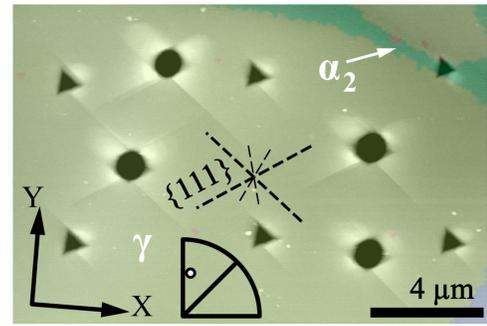
AFM characterization of the indent topography reveals the characteristic pile-up profiles of specific orientations.
