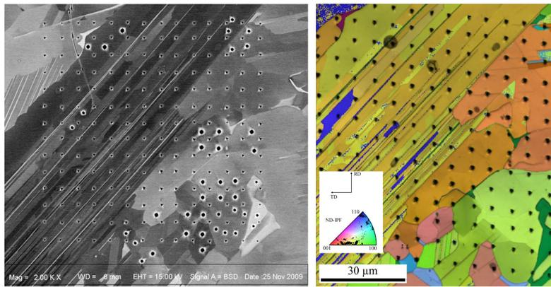
EBSD map and BSE image of a two-phase  $\gamma$ -TiAl based microstructure with indents.
