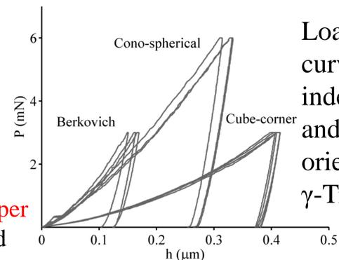
Load-displacement curves for different indenter geometries and different orientations of  $\gamma$ -TiAl.
