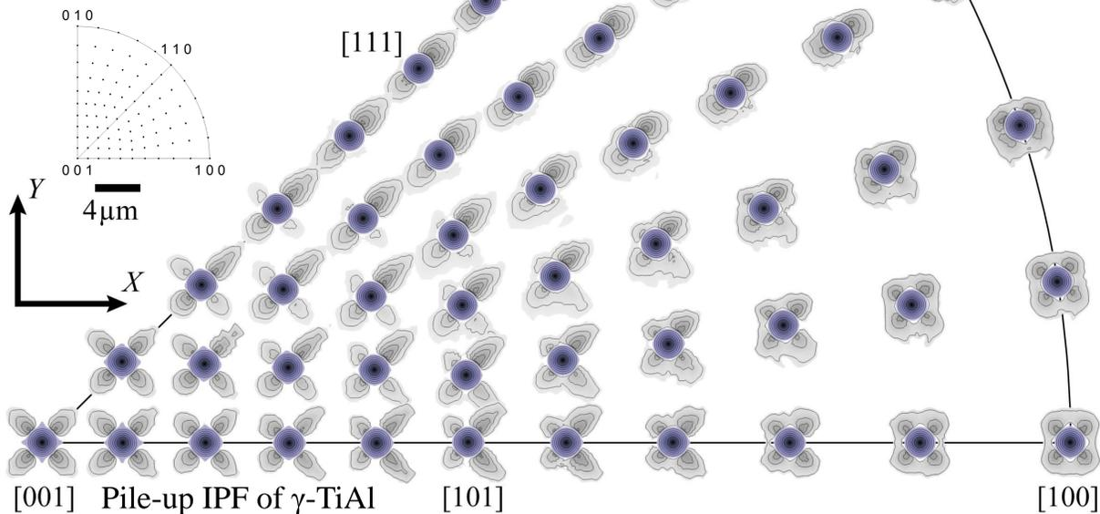
The *inverse pole figure of pileup patterns* was developed, based on a in-plane orientation convention and the representation of pile-up topographies at the stereographic projection of their indentation axis in the inverse pole figure. This graphical representation of the orientation dependent pile-up behavior can be used for any crystal structure indented with tools of arbitrary -- but preferably axisymmetric -- geometry.
