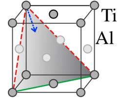
The fcc-derived  $L1_0$  structure of  $\gamma$ -TiAl; Ordinary/super dislocation glide and twinning can operate.
