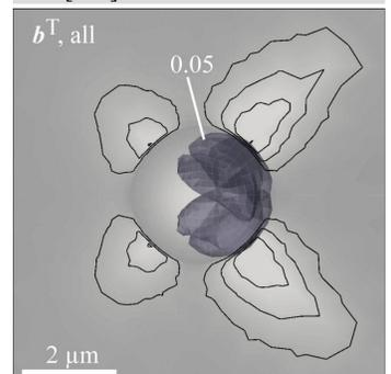
Crystal plasticity finite element simulation of the indentation process can explain the formation of the pile-up patterns based on the activation of different deformation mechanisms.
