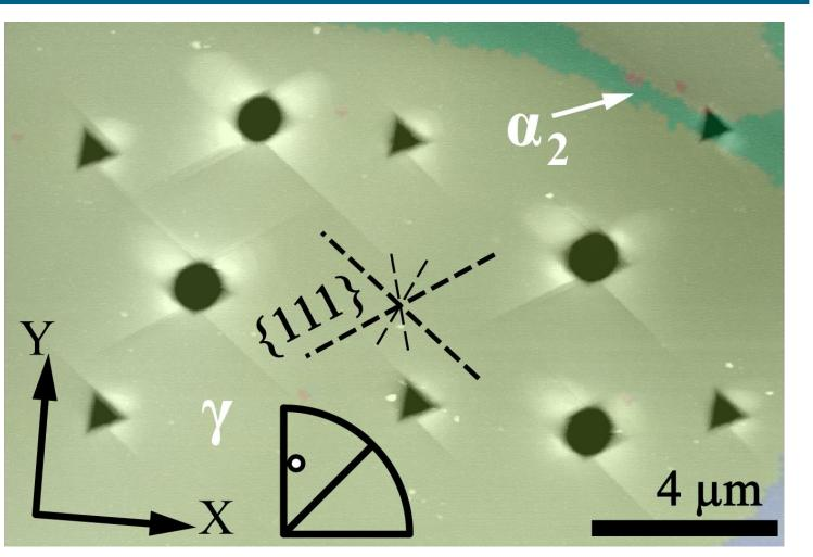
AFM characterization of the indent topography reveals the characteristic pile-up profiles
