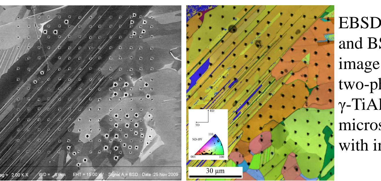
EBSD map and BSE image of a two-phase γ-TiAl based microstructure with indents.
