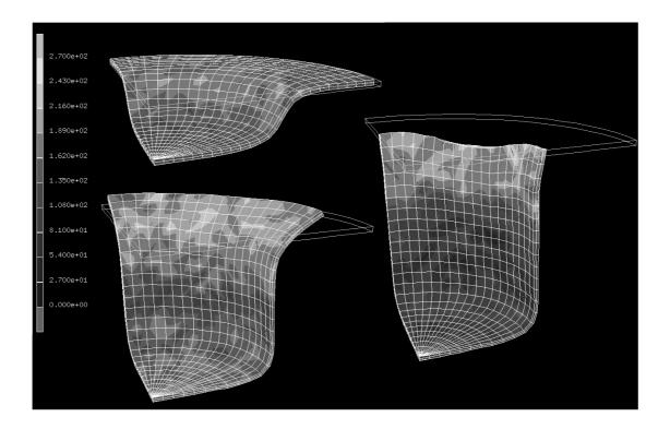
Example of a simulated large strain forming operation including crystallographic orientation information and rotation of the crystals during straining. The importance of the crystallographic texture can be seen from the resulting shape revealing the so called earing phenomenon. The simulations are elastic-plastic, i.e. spring back prediction is automatically included. The gray scale scheme indicates von Mises strains.
