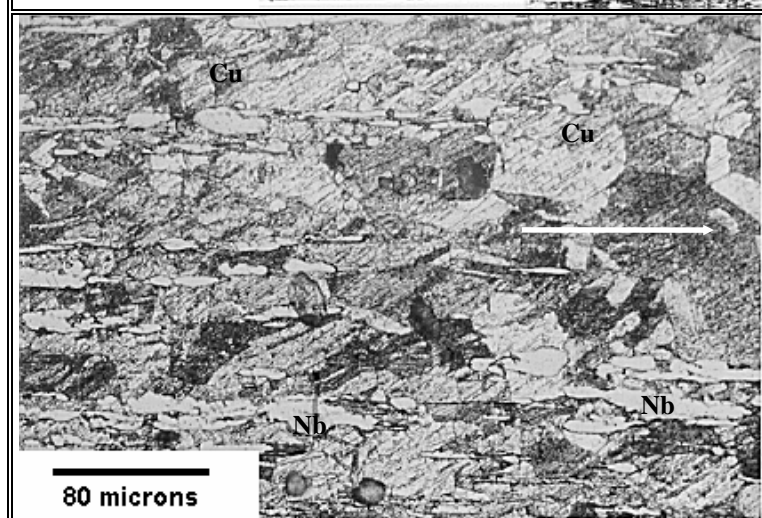
Figure B4. Microstructure of the drawn-annealed sample with \eta = 3.01 , T = 1000^\circ\text{C} , t = 12 hr on the longitudinal section. The arrow indicates the drawing direction. The recrystallized copper grains are shown with various contrasts (from light to dark shaded areas).
