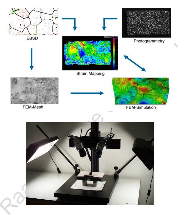
**Fig. 5a** Principle of our joint experimental procedure
