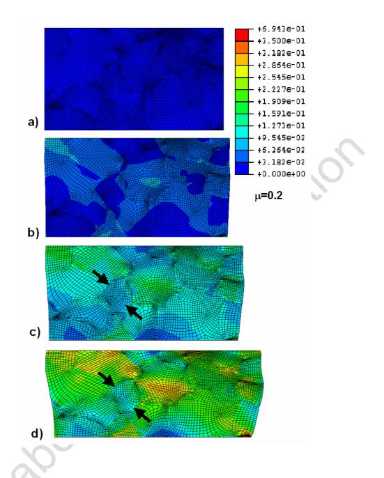
(a) The microstructure of the initial sample was mapped onto a finite element mesh. Grid configuration was conducted along the grain boundaries using a bilinear element with 4 nodes and 4 integration points (5705 elements).
