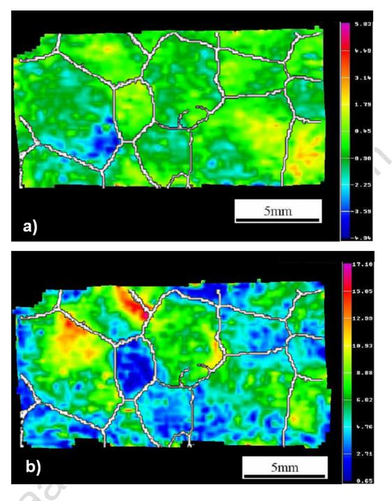
Distribution of the (a) accumulated engineering plastic shear and (b) von Mises strain in the specimen after 8% sample thickness reduction ( $\Delta d/d$ , where d is the sample extension along compression direction). The strains were determined using photogrammetry. The grain boundaries indicated by white lines were taken from microtexture measurements.
