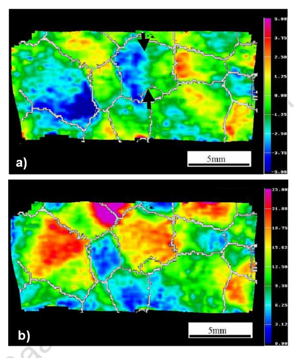
Distribution of the (a) accumulated engineering plastic shear and (b) von Mises strain in the specimen after 15% sample thickness reduction ( $\Delta d/d$ , where d is the sample extension along compression direction). The strains were determined using photogrammetry. The grain boundaries indicated by white lines were taken from microtexture measurements.
