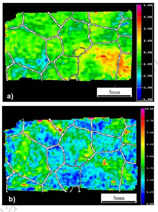
Distribution of the (a) accumulated engineering plastic shear and (b) von Mises strain in the specimen after 3% sample thickness reduction ( $\Delta d/d$ , where d is the sample extension along compression direction). The strains were determined using photogrammetry. The grain boundaries indicated by white lines were taken from microtexture measurements.
