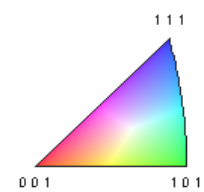
Color Coded Map Type: Inverse Pole Figure [001] Iron (Alpha)
