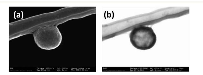
Fig. 2 Example of complementary "upper" observation of a single  $SiO_2$  submicrocapsule (about 200 nm size) onto a string of the supporting lacey carbon foil using the *In-Lens* detector (a) and in the transmission mode (b). Note the "shell-like" structure of the particle that can be visualized only in the transmission mode.
