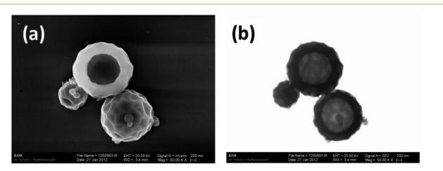
**Fig. 3** Example of complementary "upper" observation of polyepoxide-shell and oil-core particles submicrocapsules using the *In-Lens* detector (a) and in the transmission mode (b). Note the details on the outer particle surface as well as the presence of many nanoparticles in the left micrograph and the quite different occurrence of the big, bottom particle in the two imaging modes.
