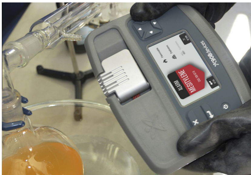
Fig. 5. M908, the world’s first and only hand-held, high-pressure mass spectrometry (HPMS) system.
