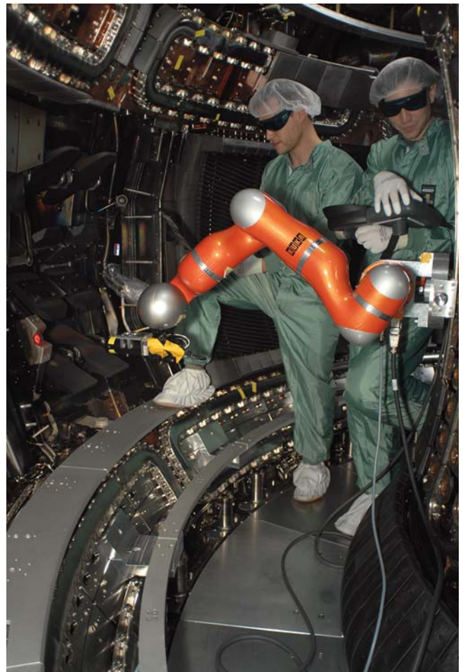
Figure 2: The LOS measurement tool IBOROB operating in ASDEX Upgrade.
