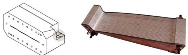
Figure 28: Left: Revised design of a helical series feed with a larger helix diameter. Right: Stacked copper and aluminium sheets of the 32-element horn array before electro-forming.
