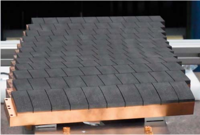
Figure 6: The plasma facing surface of the 3D machined elements mounted onto their frames.
