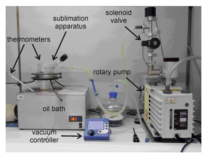
Fig. S1. Experimental setup used for the sublimation deposition of matrices
