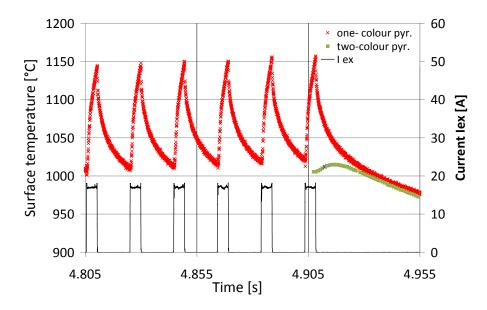
Fig. 2: Surface temperature measurement during modulated heat loading of the W lamellae. A heat flux of  $25MW/m^2$  with 5ms on/15ms periods off was applied. The extraction current  $I_{ex}$  is shown to identify the heat loading periods.
