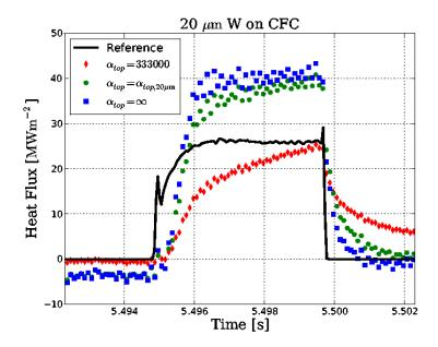
Fig. 3a, b: Comparison between the applied heat pulse (Reference) and heat fluxes calculated for (a) W-lamellae and (b)  $20\mu m$  W on CFC as example for the vertical target.  $\alpha$  is given in W·m<sup>-2</sup>·K<sup>-1</sup>.
