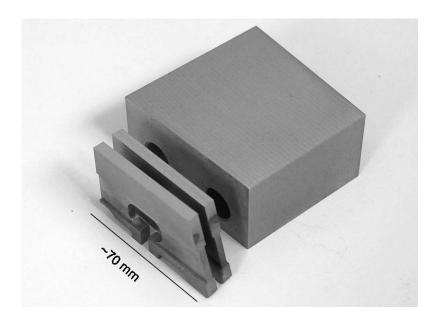
Fig. 1: Samples after loading. The W lamellae are seen in front. The 20  $\mu m$  W coated CFC tile is placed in the background.
