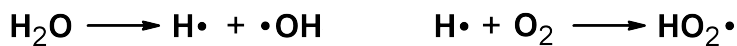
Scheme 4.3: Sonolytical dissociation of water (left) and formation of hydroperoxy radical through reaction between hydrogen radical with molecular oxygen (right).
