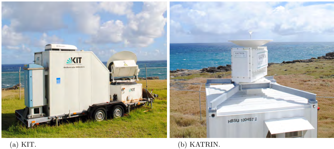
Figure 2.4: Images of the two cloud radars, used in this study (a) KIT and (b) KATRIN. (Courtesy: Friedhelm Jansen)
