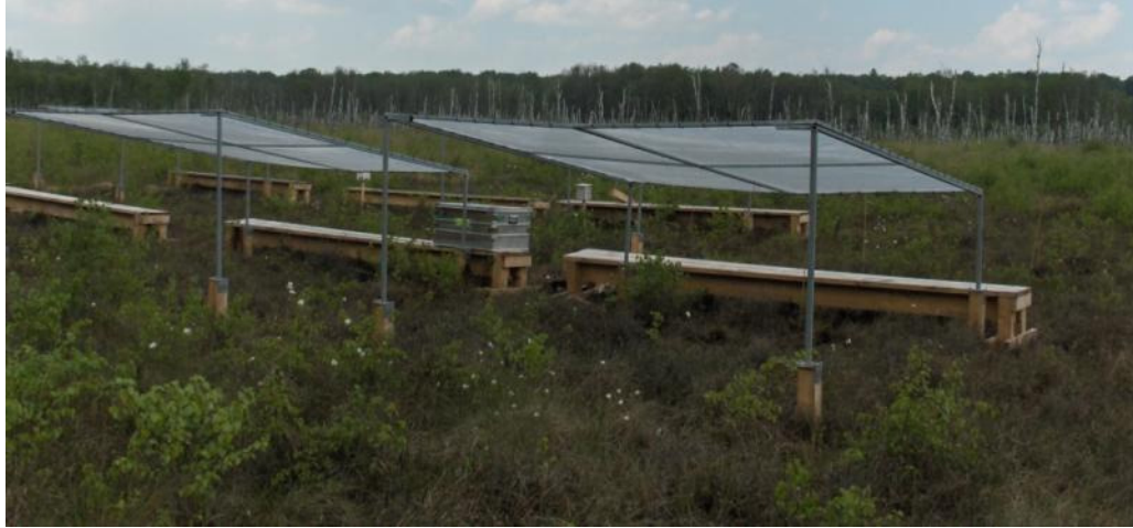
Figure 8: Rainout shelters at the heath subsite in the Himmelmoor.
