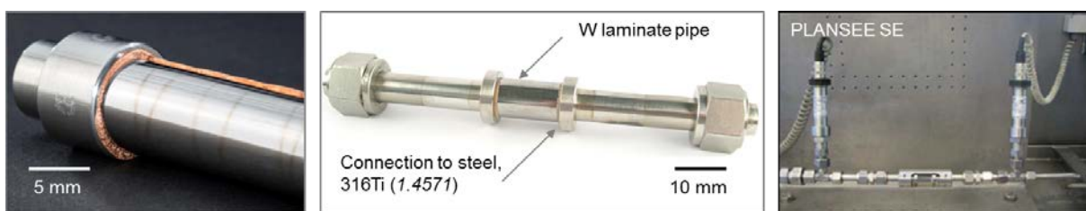
Fig. 6. Left: Tungsten laminate pipes can be joined to austenitic steel (1.4571) and burst test samples and HHF test samples can be produced. Middle: This picture shows the burst test sample after the test. The pipe shows no residual damage after 1000 bar at RT. Right: Test configuration and burst test device at PLANSEE SE.
