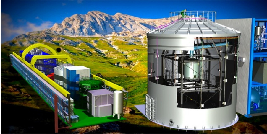
Figure 1.6: Sketch of the XENON1T experiment [22]. Left: Hall B at LNGS, where XENON1T is being constructed at the time of writing. Right: The water tank with the two-phase xenon TPC inside.
