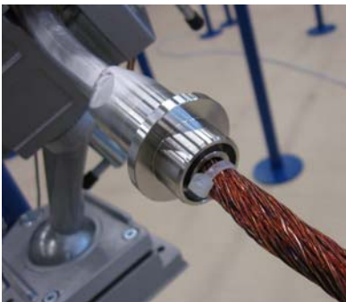
Fig. 7. Transition piece at the bus bar end
