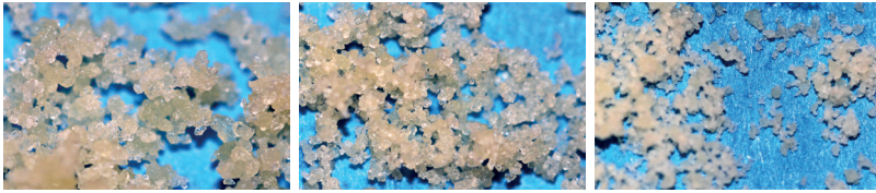
(a) 15 wt% oleosomes, air: 439 L/h, liquid: 0.3 L/h, T_{in} = 100\text{ }^{\circ}\text{C} (b) 15 wt% oleosomes, air: 1052 L/h, liquid: 0.3 L/h, T_{in} = 100\text{ }^{\circ}\text{C} (c) 15 wt% oleosomes, air: 1052 L/h, liquid: 0.16 L/h, T_{in} = 100\text{ }^{\circ}\text{C}
