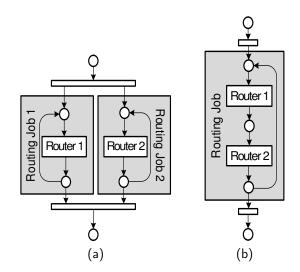
Figure 1: Asynchronous (a) vs. synchronous (b) control flow
