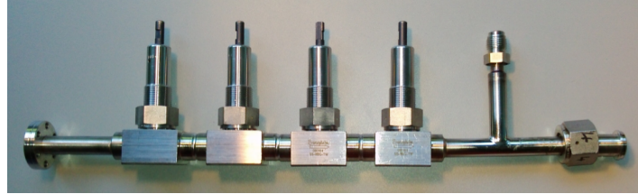
Figure 3.3.: A standard xenon sample pipette used in this work. Four fully metal sealed valves are welded together and enclose three separable sub-volumes. The innermost volume is thus shielded on both sides by two valves and one buffer xenon volume minimizing the impact of eventually internally leaking valves.
