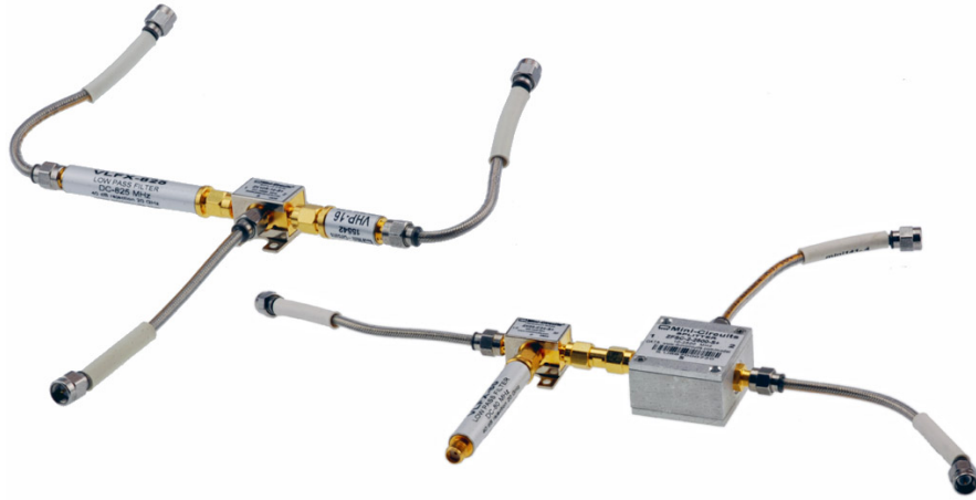
Figure 7.7: Implementation of FDS auxiliary functions. Left: modulation combiner, right: reference oscillator mixer.
