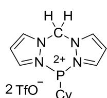
CyPCl<sub>2</sub> (0.26 mL, 1.7 mmol) and TMSOTf (0.61 mL, 3.4 mmol) were added at –78°C to a suspension of [H<sub>2</sub>C(Pz)<sub>2</sub>] (**8**) (250 mg, 1.7 mmol) in CH<sub>2</sub>Cl<sub>2</sub> (5 mL) and the mixture allowed to warm up to room temperature overnight. The solvents were then evaporated in vacuum, the residue dissolved in CH<sub>3</sub>CN (2 mL) and Et<sub>2</sub>O (10 mL) was added to precipitate the product. White solid (433 mg, 46%).
