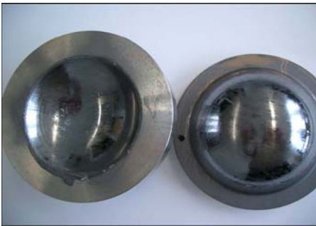
Fig. 13. Test 19/ ball and cup after 1000 strokes.
