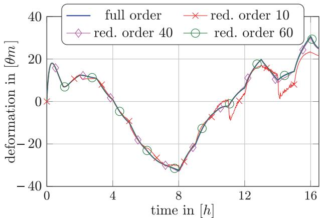
**Figure 3:** Displacement evolution of the full order system compared to ROMs of order  $r = 10, 40$  and  $60$ .
