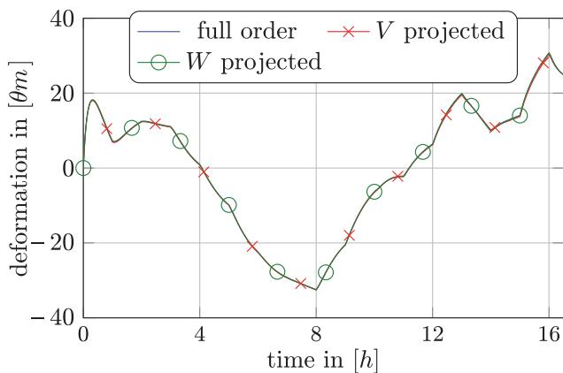
**Figure 6:** Displacement evolution of the full order system compared to the ROM of order  $r = 75$  generated by input ( $V$ ) or output ( $W$ ) Krylov subspaces, respectively.
