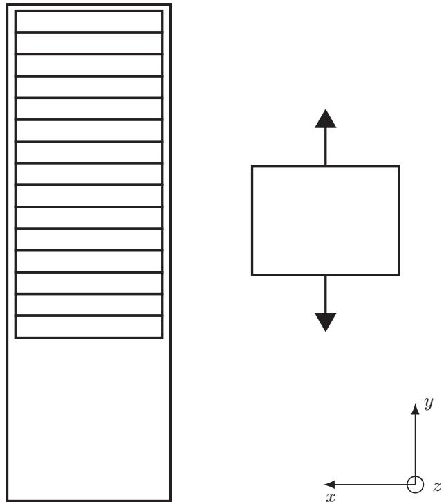
Figure 2: Scheme of partitioned guide rails and moving slide.
