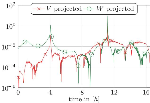
**Figure 7:** Relative error of the reduced order models of order  $r = 75$  in time domain.
