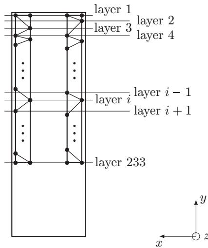
**Figure 5:** Parameter affine splitting based on horizontal layers with same  $y$ -coordinates of FE nodes.
