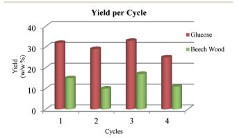
Fig. 2 Levulinic acid yield per cycle during recycling experiments of the acidic aqueous phase for the hydrolysis of glucose and beechwood.
